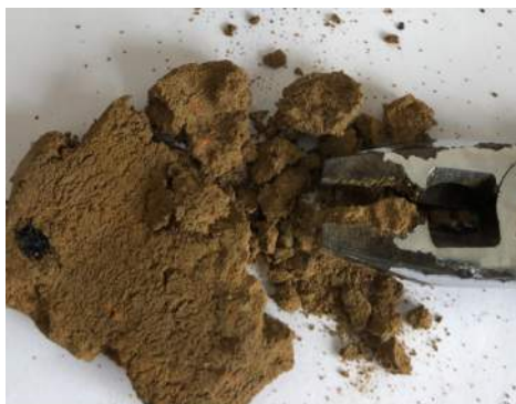
Test 2 - Took pliers to break the sample, the finger pressure in effective on smaller pieces.
